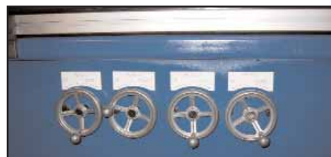
Hand wheels are used to raise and lower the screw jacks
