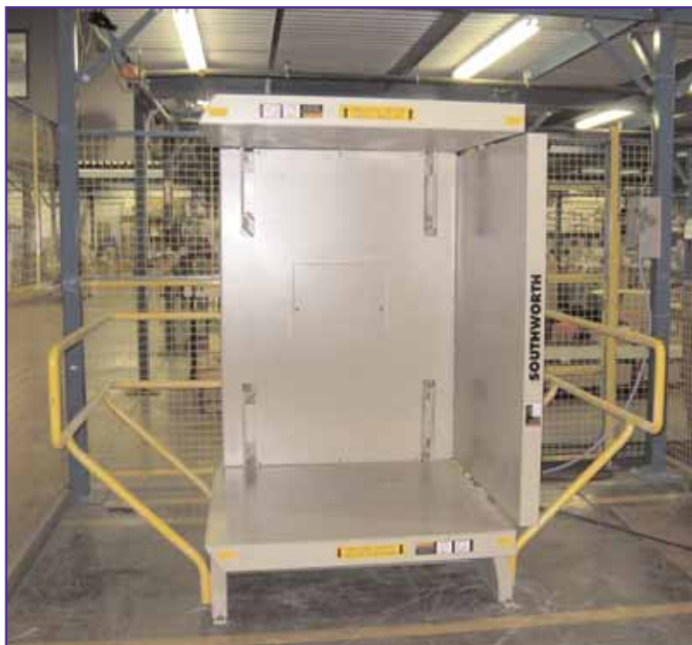
The PalletPal Rotator/Inverter takes approx. one minute to complete an entire cycle (180 degrees)
